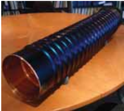
Fig 5. Spectral layer on copper tube
