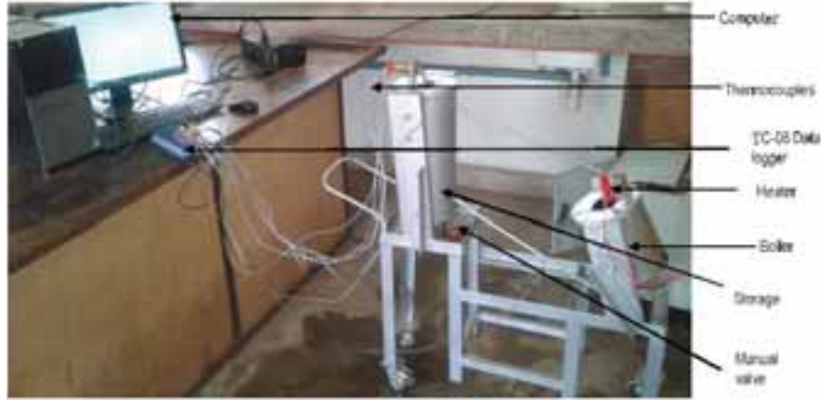
Fig. 2: A self circulating system consisting of a storage tank and a boiler. Sunflower oil was used in the boiler and the three types of oil were put in the storage tank one after the other. The storage was filled with each type of oil and this got heated in the boiler and thereby charging the storage.
