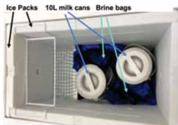
Fig. 2: PV Powered Chiller Using Thermal Ice Storage and Brine Bags to Chill Evening Milk
