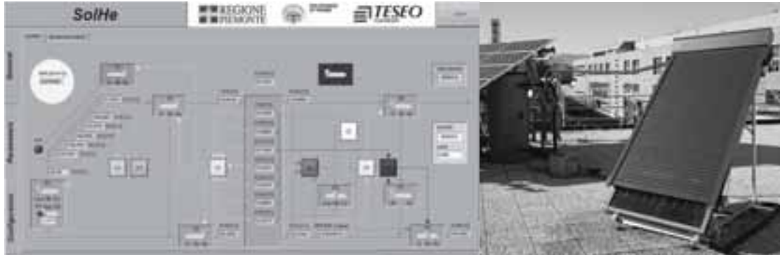
Fig. 3: Left: schematic of the analysed PCS-based solar thermal system. Right: the full scale prototype at Politecnico di Torino.
