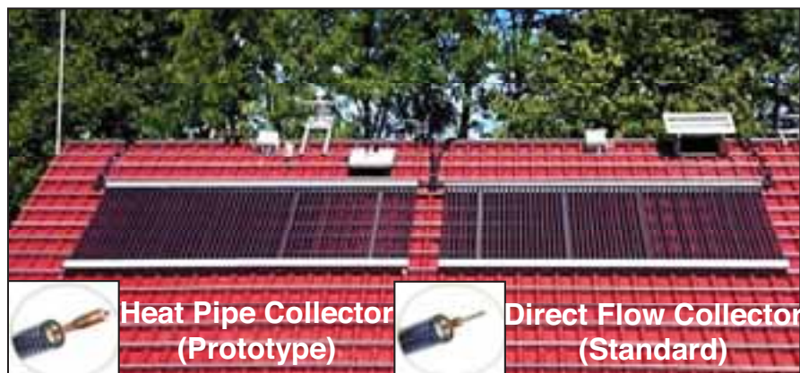
Fig. 2: Test roof with both prototype and reference evacuated tube collector fields
