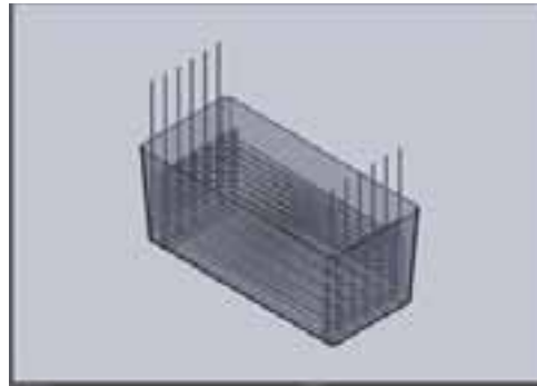
Figure 14 Schematic drawing of the storage container and the heat exchanger
