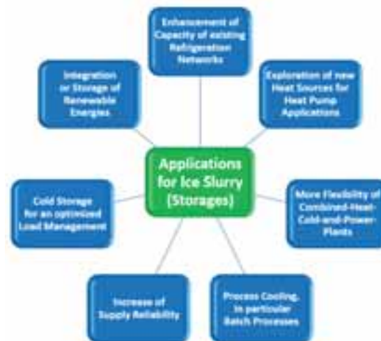
Fig. 3: General fields of application for ice slurry as secondary refrigerant and storage medium
