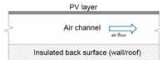
Fig. 1: Typical PV/T configuration
