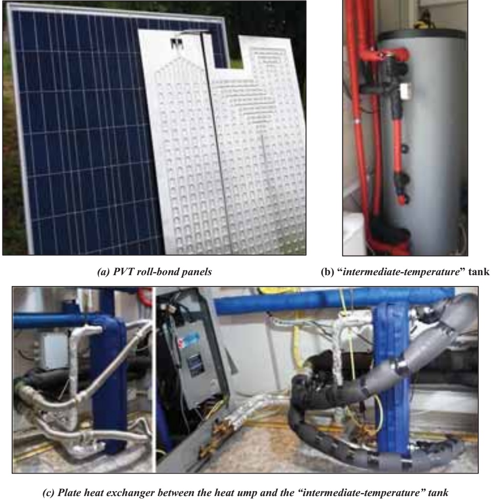
Fig. 3: Details of the experimental setup
