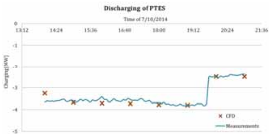
Fig. 13: Measured and CFD predicted discharge power of the PTES for the discharge case on October 7
