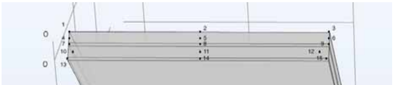
Figure 4 : Measurement points on the air outlet of the collector
