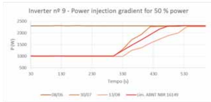
Fig. 9: Power injection gradient evaluation results for inverter n° 9 with 50 % rated power.
