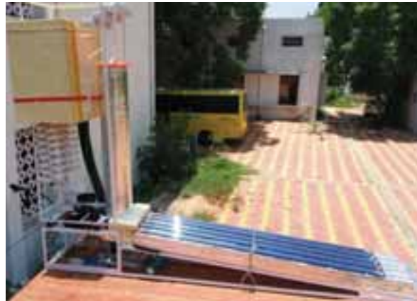
Fig. 2: Solar-Polar DAR demonstration system with heat pipe solar collector array, installed at Anna University campus, Chennai.
