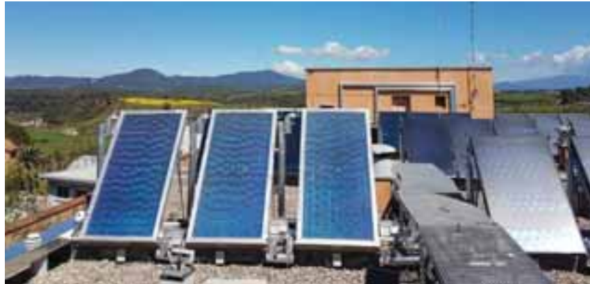
Fig. 12 Solar energy capturing field of the Albada Building in Parc Tauli Hospital. The three prototypes are tested alongside the conventional flat plate solar collectors without TIM.
