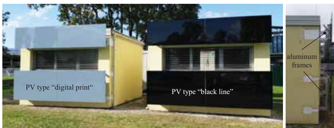
Figure 8: Test boxes with installed aluminum frame and the photovoltaic modules, the right box is the test facility with the installed cooling system while the left box is used as reference box (Source: TU Graz)
