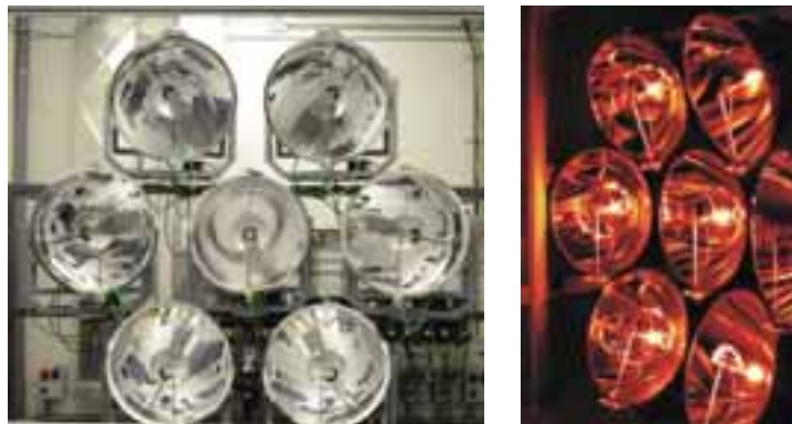
Fig. 1: Left, frontal photograph of the high flux solar simulator. Right, attenuated photograph of the Xenon lamps in operation
