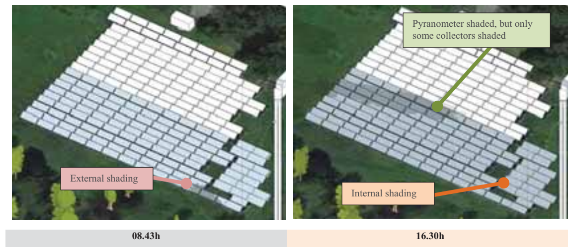
Fig. 4: Irradiance analysis of the test plant (2017-09-27)
