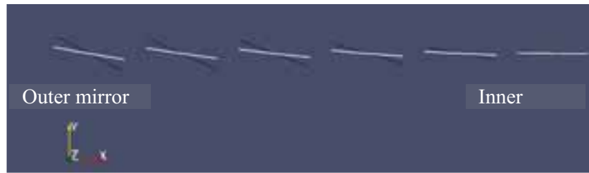
Fig. 3 Orientation of mirrors at noon. Blue mirrors: receiver height of 2m. White mirrors: receiver height of 8m. Taking into account that solar radiation at noon comes in Y direction (with some amount of Z component), clearly the higher the receiver is placed, the more effective area the mirrors present to the solar radiation. This effect is more important for the outer mirrors.
