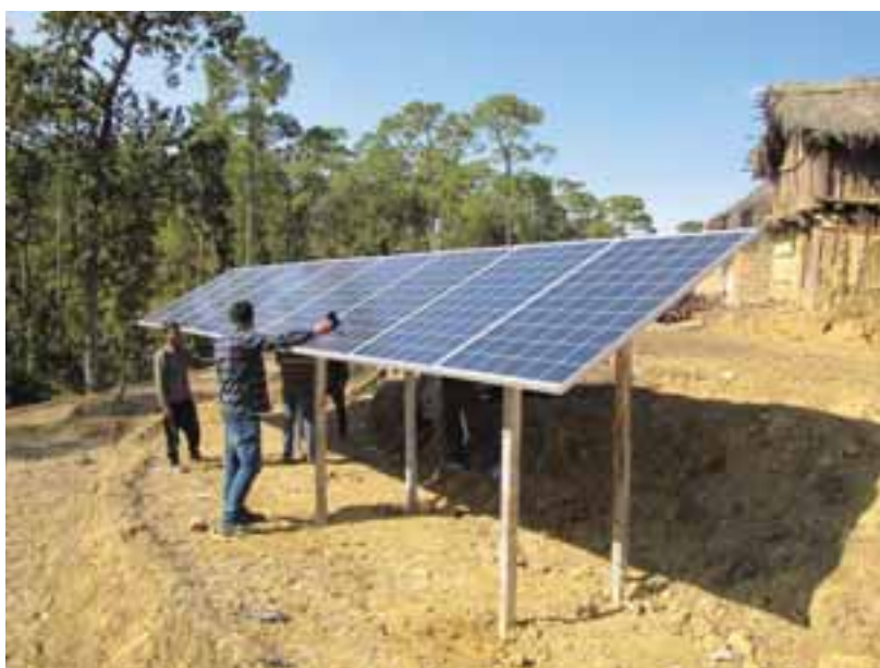
Figure 12: WI technicians measuring solar irradiance for the PVWP installed in Odaltal village of Surkhet District.
