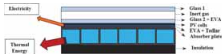
Fig. 2: Schematic diagram of the novel PVT collector proposed in this work, based on a polycarbonate flat-box structure.
