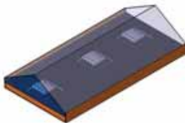
Figure2, Sample geometrical modeling of solar tunnel dryer.
