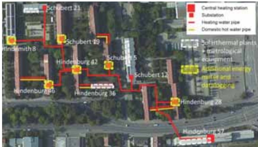
Fig. 2: Scheme of the existing district heating network with decentralized solar thermal plants
