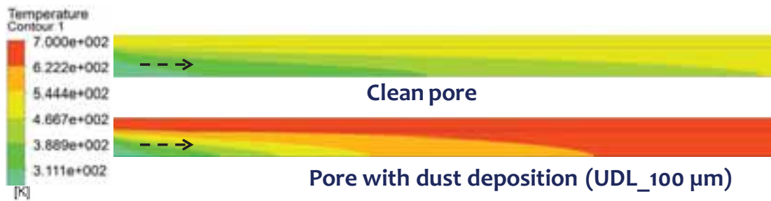
Fig. 7: Temperature contours for a clean pore and for a partially blocked with uniform dust layer (UDL) thickness of 100 \mu\text{m} and the applied uniform heat flux along the pore length
