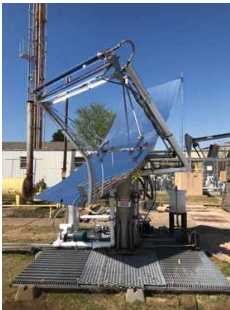
Figure 8 Prototype hybrid CSP-CPV system in on sun operation
