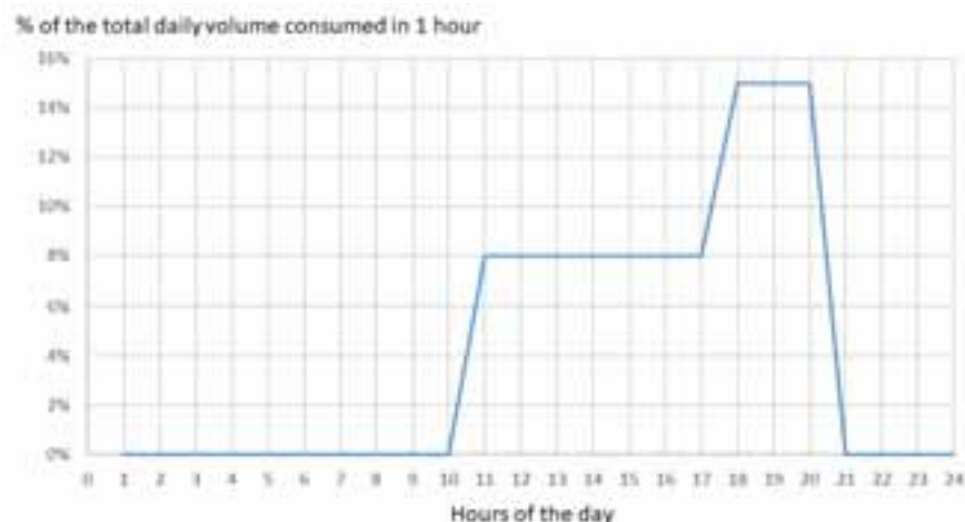
Fig. 5: Hot water need profile in the simulation
