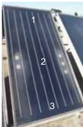
Fig. 2: STC with zinc reference materials and the indication where environmental contaminants were collected after dismantling of collectors
