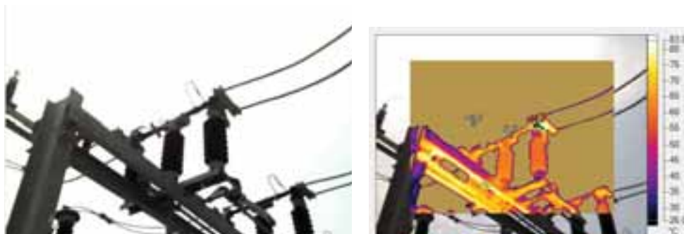
Fig 8: Visible and infrared image of isolator and bus bars.
