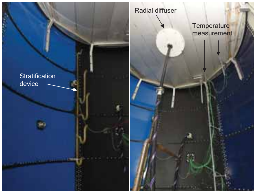
Figure 7: Stratification device (left), radial diffuser with flexible EPDM-hose and temperature measurement probes (right), February 2017
