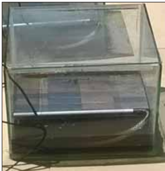
Plate 2: Fabricated photo catalytic effluent treatment unit
