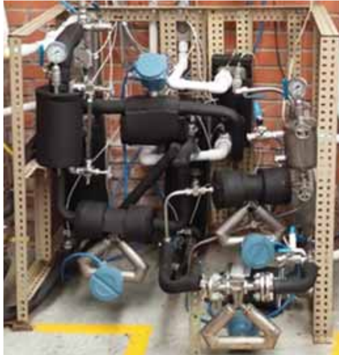
Fig. 3: Developed absorption cooling machine
