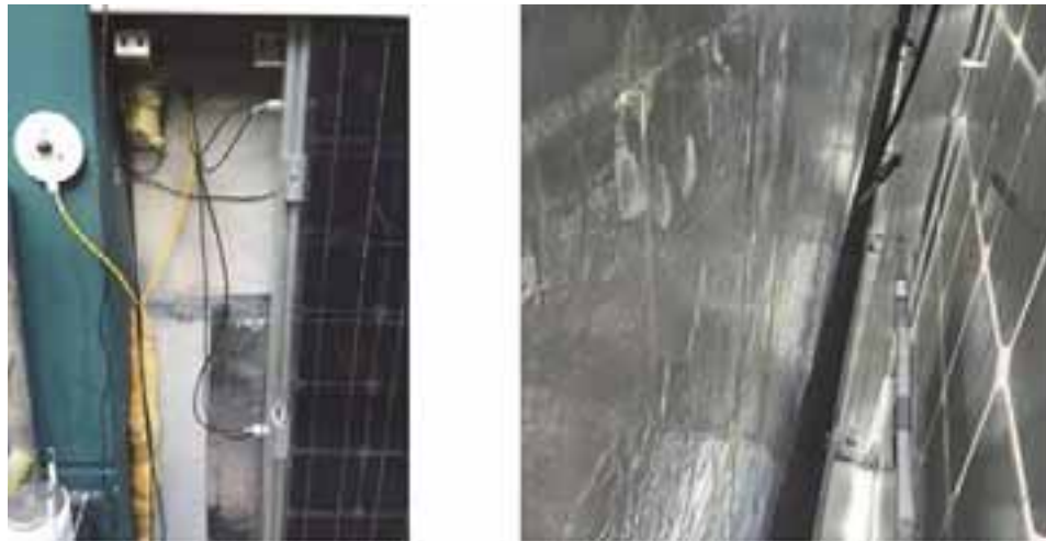
Fig. 6 Pyranometer and outdoor temperature sensor (left), anemometer and inner temperature sensors (right).
