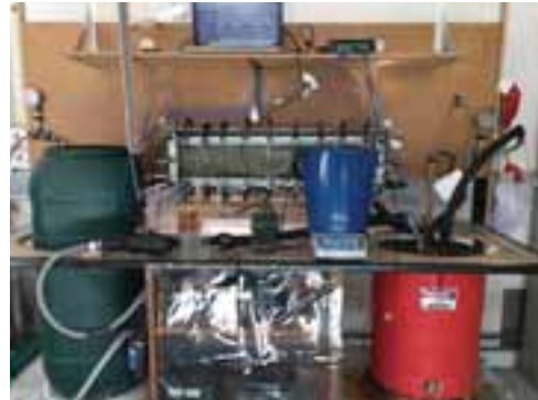
Fig. 2. Left: Schematic diagram of the MD experimental setup; Right: Actual indoor lab scale PGMD experimental setup
