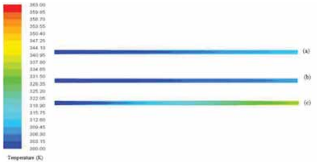
Fig. 9: Temperature contours for (a) Therminol, (b) Water, (c) NaK78 at 0.5 kg/sec mass flow rate with non-uniform heat flux
