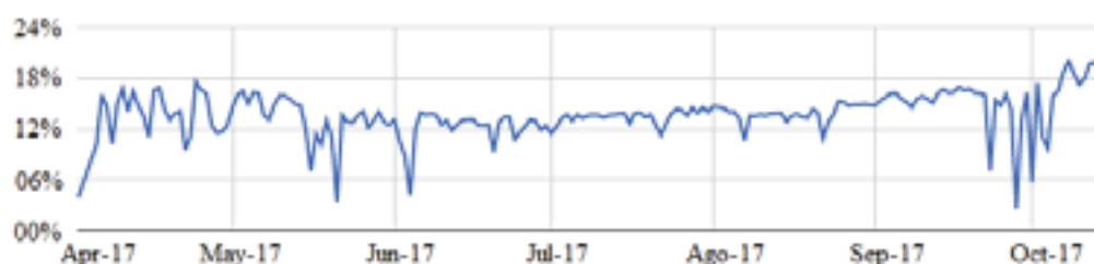
Fig. 10: Curve of daily capacity factor values observed on 34 kWp grid-connected PV system from April to October 2017.
