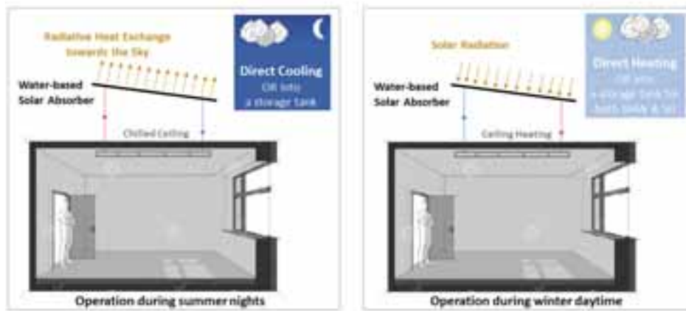
Fig. 2: Energy supply system that provides space cooling in summer (left) and space heating in winter (right)
