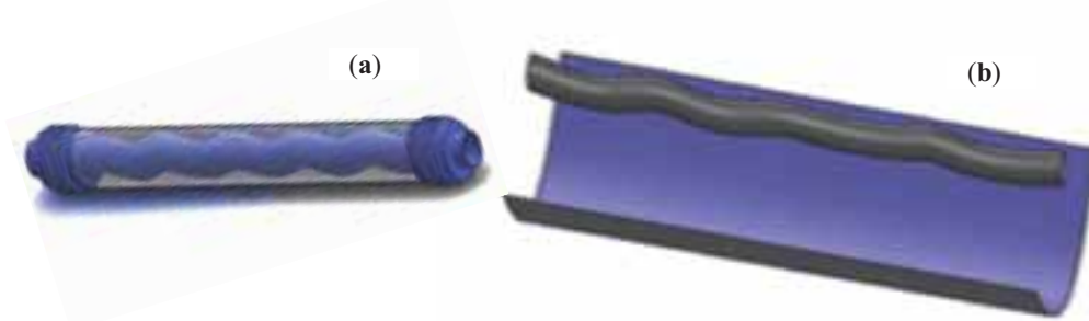
Fig. 1: (a) The novel undulated PTC receiver. (b) A PTC module with the novel undulated absorber.
