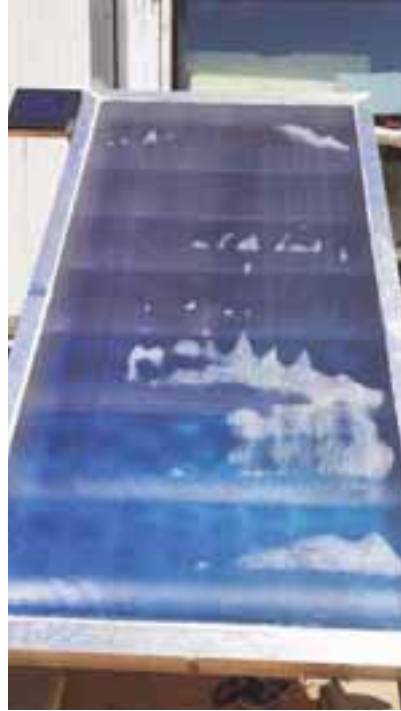
Fig. 8 Condensation phenomenon observed in a preliminary prototype
