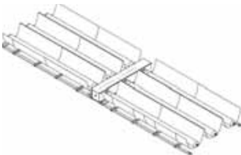
Figure 9 – Final E/W XCPC collector prototype. 6 CPCs are plumbed off a centralized manifold box.
