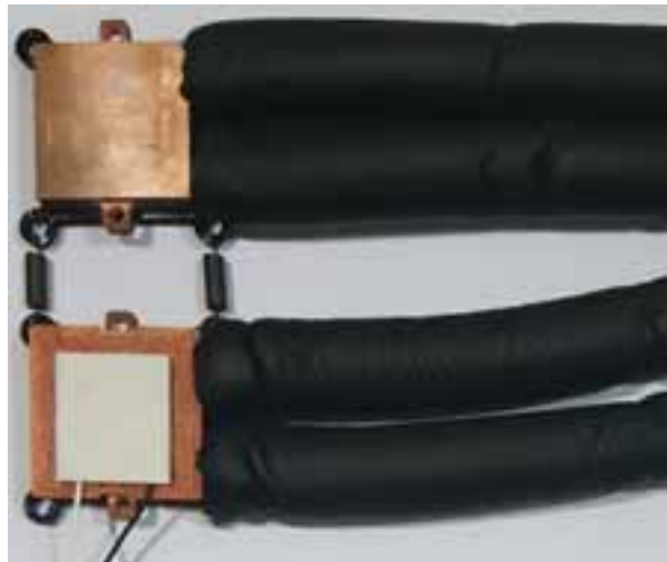
Figure 6 the TEG installed on one side of the water blocks.
