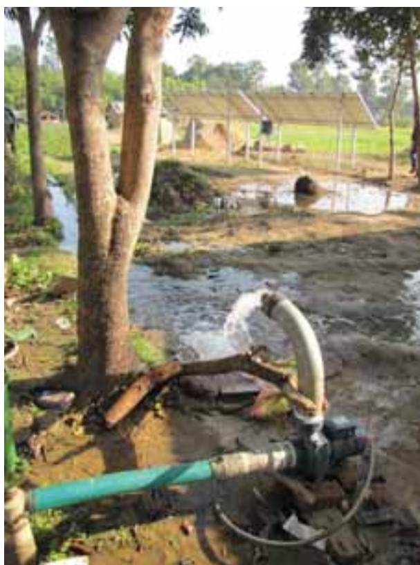
Fig. 4: Flood irrigation via a surface centrifugal solar water pump managed by Phattu Tharu of Bansgadhi, Bardiya.
